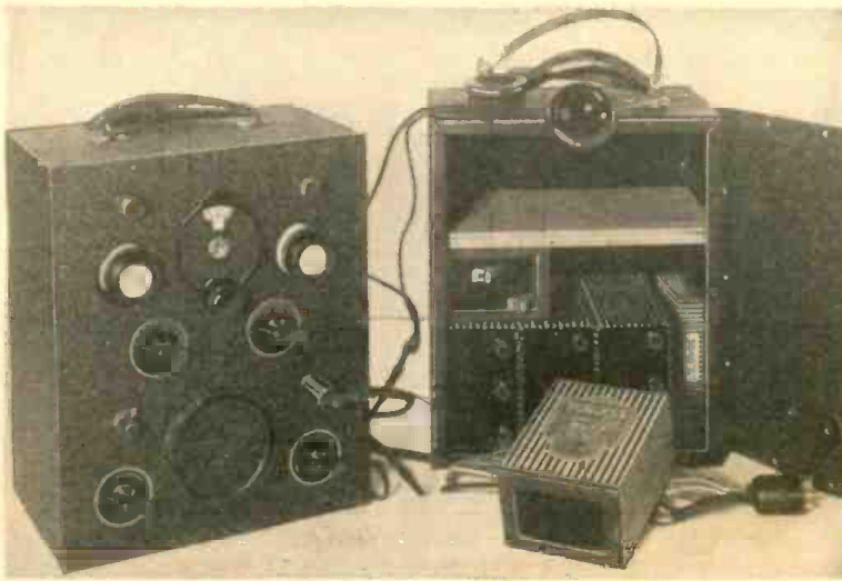
This is one of the finest all-wave portable sets that we have seen. The weight is divided by placing the batteries in a separate cabinet.
