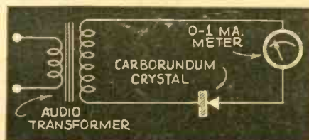
A crystal detector and a low-range milliammeter, and you have an excellent output and signal-level meter.
