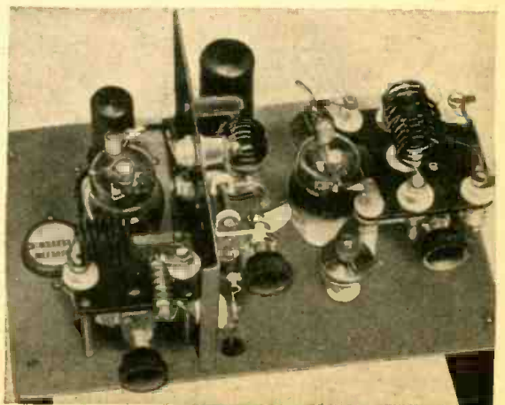
Fig. D. This "prof." looking 18 watt, 5 meter transmitter will interest every "Ham"; it's perfectly stabilized by crystal control.
